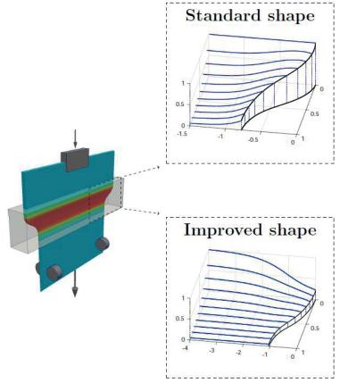
Above. Mathematical model prediction for the evolution of a rectangular glass preform as it is stretched and drawn in a redraw furnace. The resulting sheets have thick edges. In the lower right panel we begin with an optimally shaped glass preform for which the final sheets have uniform thickness. Right. Randomly arranged obstracles in a filter (right) lead to channel flows that improve performance compared with periodic arrangements.
