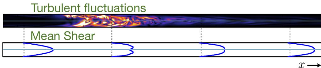
Figure 1: Transition to turbulence in a pipe flow
