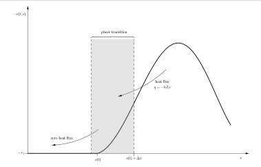
• Flow of energy (heat flux) in the liquid is  $q = -k\partial_x v(t,x)$
