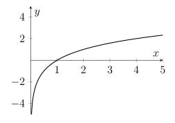
• The graph of y = f(x - a) is the translation of the graph of y = f(x) by a distance a in the positive x-direction.
