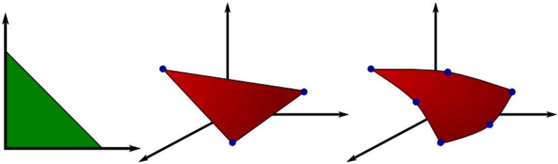
**Figure:** Examples of different surface finite elements in the case  $n = 2$ . Left shows a reference finite element (in green), centre shows an affine finite element and right shows an isoparametric surface finite element with a quadratic  $F_K$ . The plot shows the element domains in red and the location of nodes in blue.
