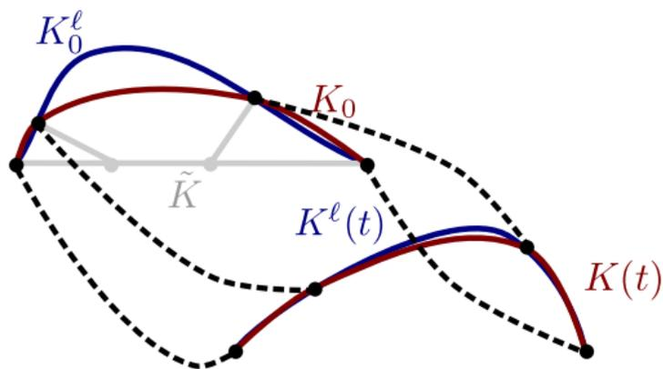
**Figure:** Examples of construction of an isoparametric evolving surface finite element for  $k = 3$ . The Lagrange nodes  $a_i(t)$  follow the dashed black trajectories from the initial element  $K_0 \subset \Gamma_{h,0}$  to a element  $K(t) \subset \Gamma_h(t)$ .
