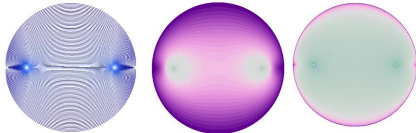
**Figure 2:** Flow streamlines indicate all regions of the dish are reached. We see that velocity is slightly higher through the middle channel. However, on a log scale, we see that only the edges form stagnant regions
