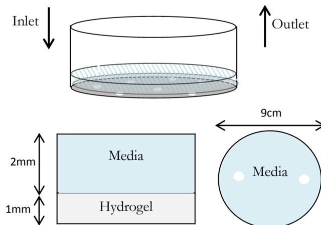
**Figure 1: Bioreactor setup.** Organoids are suspended in layer of hydrogel below a layer of culture media. Media is replenished via flow across the dish.
