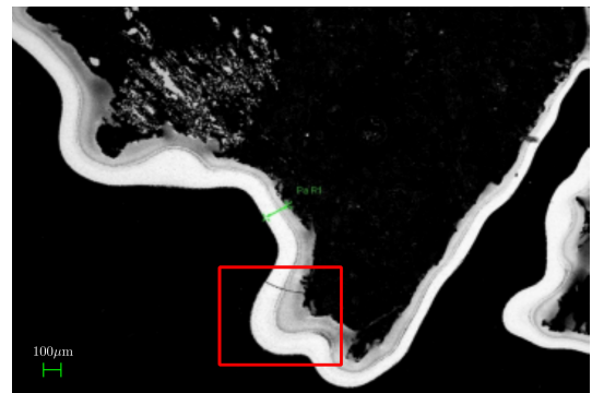
Figure 1—Electron microscope image of the condensate. The dark upper region is a particle of charge, and the white layer is the condensate.
