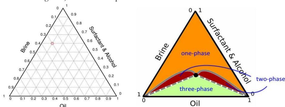
Figure 3: Ternary diagrams for a surfactant-oil-brine (SOB) system. (left) The coordinate system. The point that is marked in red has volume fractions (Surfactant & Alcohol, Oil, Brine) = (0.6, 0.1, 0.3). (right) The standard empirical understanding of a typical output for a ternary phase diagram. Colours are used to indicate systems with different number of phases.
