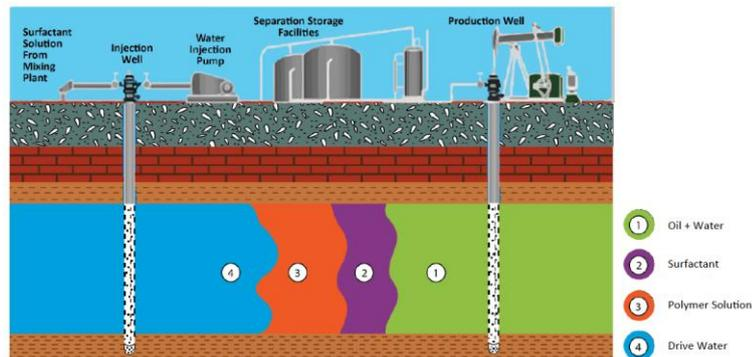
**Figure 1: Schematic diagram of an oil reservoir. An oil recovery mixture is injected underground to mobilize the oil that is trapped.** Source: Primera Reservoir
