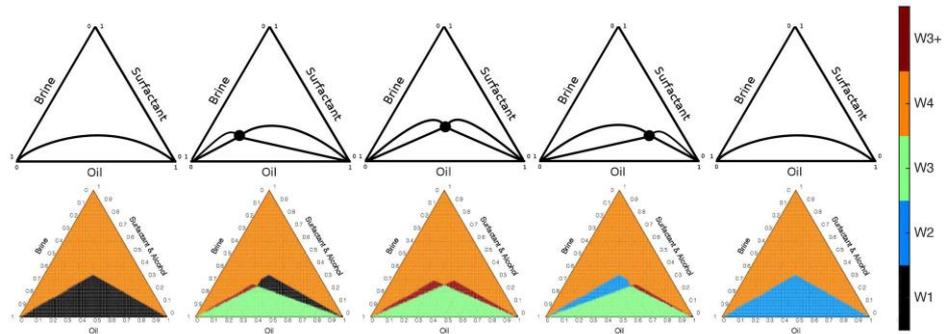
Figure 4: Typical ternary phase diagrams with salinity increasing from left to right, when alcohol is absent. Schematic diagrams along the top row indicate the expected behaviour [2], with solid lines indicating that adjacent regions differ in the number of phases and black circles indicating the central point of each diagram. The bottom row displays predictions with the HLD-NAC model. Colours indicate different Winsor schemes, as shown in the colour bar.
