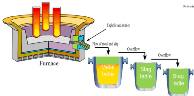
Figure 1: A schematic of the tapping process in ferromanganese production, from [1].
