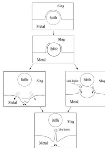
a) Diagram showing how metal droplets impacts can be formed by rising air bubbles. [2].
