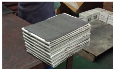
Figure 1: A single lead-acid cell (Photo: Ashley Grealish, BBOXX). Alternating positive and negative electrodes; soldered together in parallel to make two large electrodes. A (12V) battery is made up of six (2V) cells connected in series.
