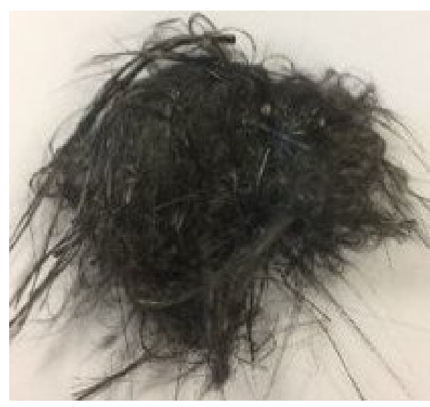
Figure 2 – A photo of a web of carbon fibres before carding.
